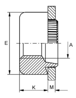
Female thread A = M14Height K = 10.0Outer diameter E = 25.0Plate thickness = 2.3 to 2.5
